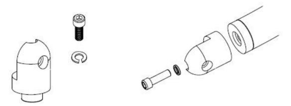
At the other end of the rear leg insert 1 x threaded fitting with the raised circle base of the fitting into the counter sunk area at the end of the short leg. Use the M12 bolt and split washer inserted through the center and tighten. Repeat this process to the other rear leg.
