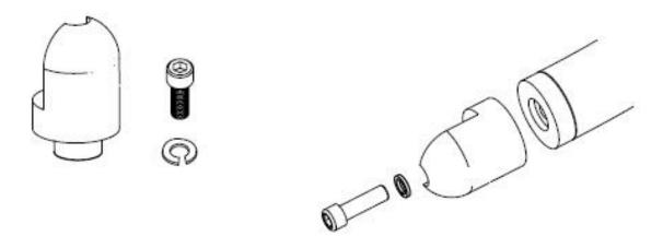
Step 5: Assembly of Deck Mount Reference
