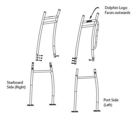
STEP 4: Attach the ball clamps to top of Side Frames
