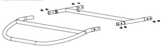
STEP 6: Attach the Side Supports to the Assemble Top Section
