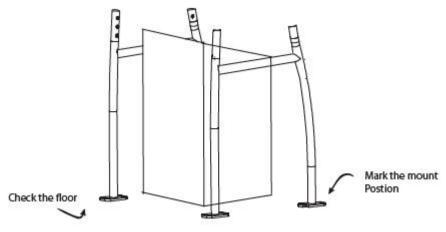
STEP 3: Assemble the side support frame
